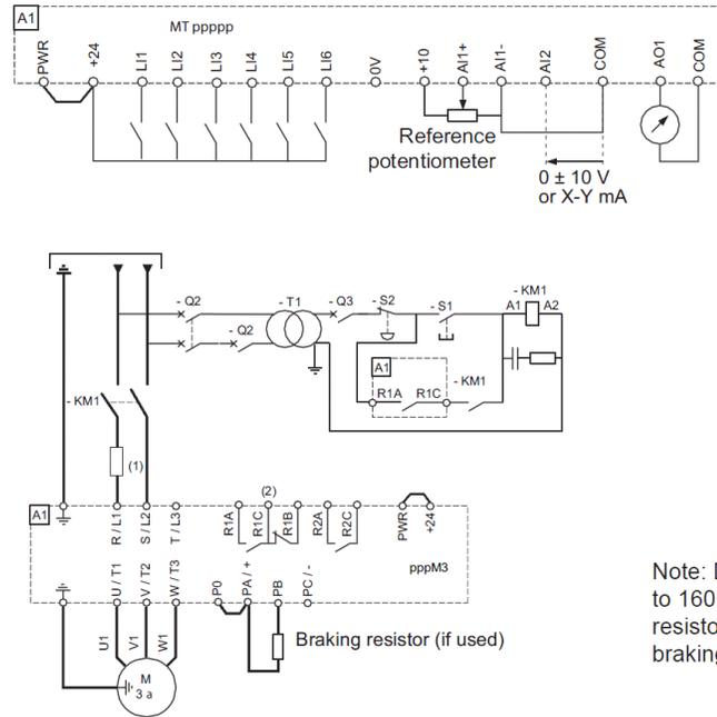
Note: Diagram applies to models rated up to 160 kW (250 HP). Above this, braking resistors are connected to an external braking module.
