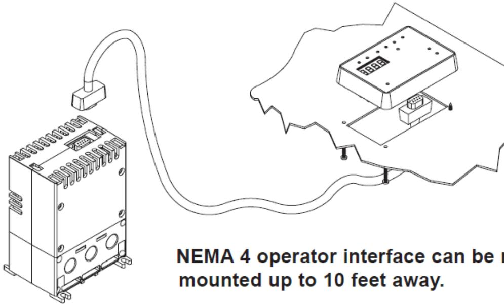
**NEMA 4 operator interface can be remote mounted up to 10 feet away.**
