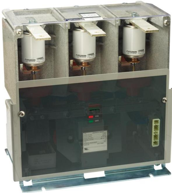
Motortronics MVF Series 7.2kV Class, 'Non-Latching' and 'Latching' Series of medium voltage three-phase vacuum contactors can be used in power systems with a rated voltage up to 7.2 kV and can be used for continuous AC operating currents of up to 400 amperes. Control voltage for the contactor is AC/DC 100~125V or AC/DC 200~230V\*, including an auxiliary relay with 3 NO and 2NC contacts.
