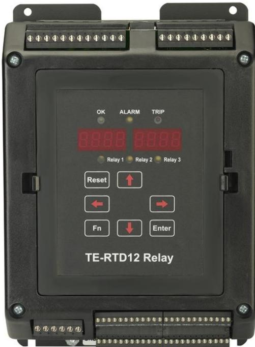
The TE-RTD12 Relay device adds advanced RTD and Current monitoring capability to your new or existing motor system. The TE-RTD12 Relay device offers 12 built-in RTD inputs, 3 programmable output relays (5A), 2 isolated analog inputs (4-20mA), 3 isolated digital inputs, 1 isolated analog output (4-20mA) and differential current feedback monitoring.
